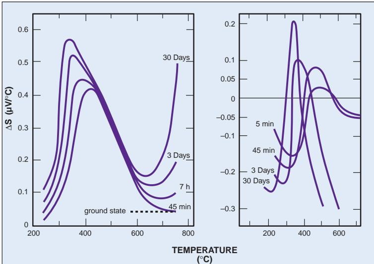
FIGURE 3 (Left). Changes in the Seebeck coefficient ( $\Delta S$ ) of a typical type KP thermoelement vs. platinum on initial heating, as a function of constant aging temperature for the indicated times (Ref. 3).
